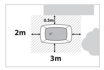
leave 0.5m space around system for care and maintenance (total 2m by 3m required)
