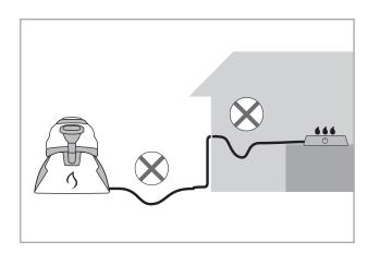
there should be no U-shaped bends in the gas tube to prevent water vapor accumulation
