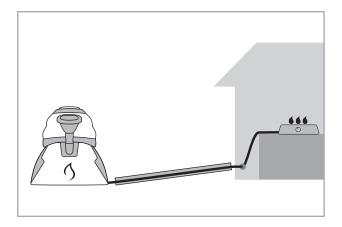
gas tubing should be raised at an angle from system to stove.
