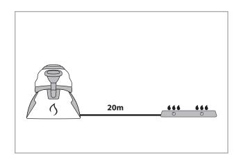
system can be connected to stove/appliance up to 20m away (10m gas tubing provided)
