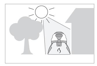
system should be in a sunny area for optimum gas production
